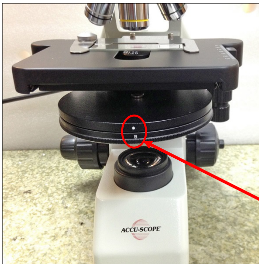
Front Turret Installed and Positioned Currently in Optic Axis
