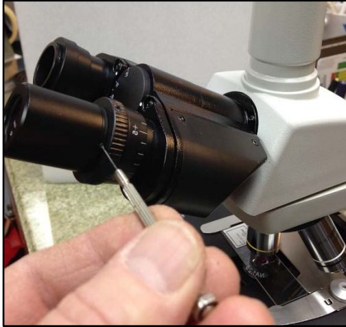
Loosen the Set Screw on Eyepiece
